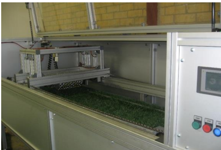
Figure 6: Lisport wear tester. (Reproduced with permission from Tapex)
