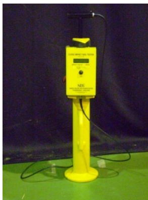
Figure 7: Clegg hammer for measuring ground hardness by impact force.
