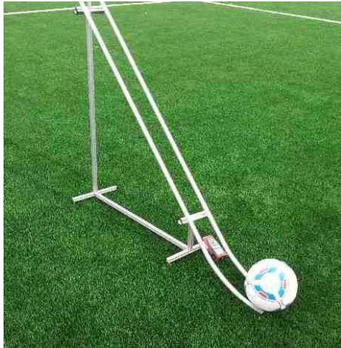
Figure 11 : Ball roll test set-up for calibrated round ball
