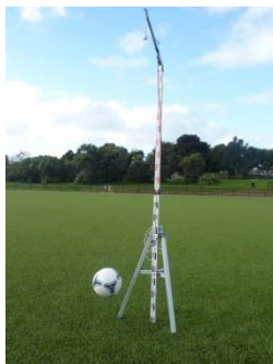
Figure 12: Vertical ball rebound test equipment.
