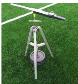
Figure 10: Studded Boot Apparatus for measuring rotational traction.
