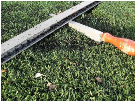
Figure 14: Photo of a Straight Edge used to measure surface evenness.
