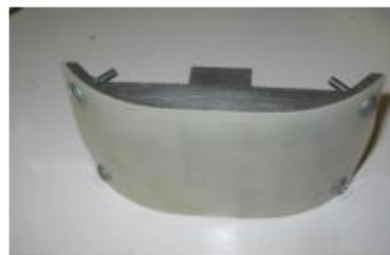
Figure 9: Securisport test foot with skin attached. (Reproduced with permission from FIFA and IRB)
